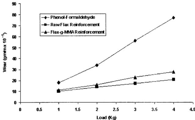
**Figure 3.** Effect of raw flax and flax-g-poly(MMA) reinforcement on wear rate of the phenol-formaldehyde composites.
