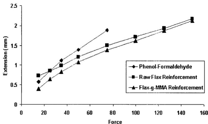
**Figure 4.** Effect of raw flax and flax-g-poly(MMA) reinforcement on tensile strength of the phenol-formaldehyde composites.
