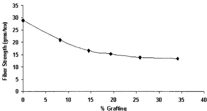
Figure 1. Effect of % grafting on fiber strength.
