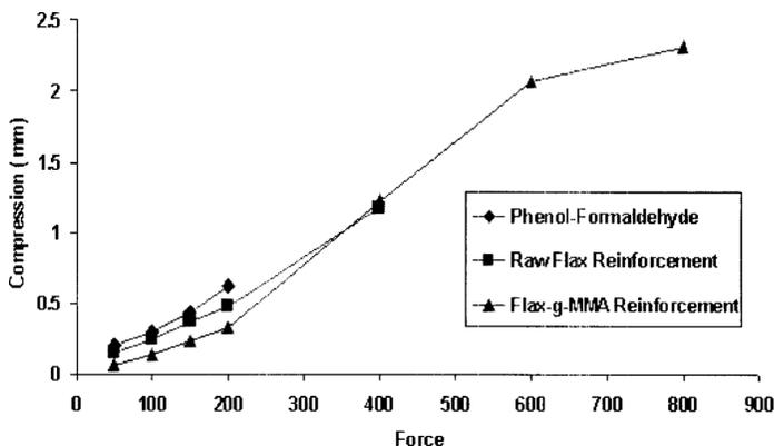
**Figure 5.** Effect of raw flax and flax-g-poly(MMA) reinforcement on compressive strength of the phenol-formaldehyde composites.
